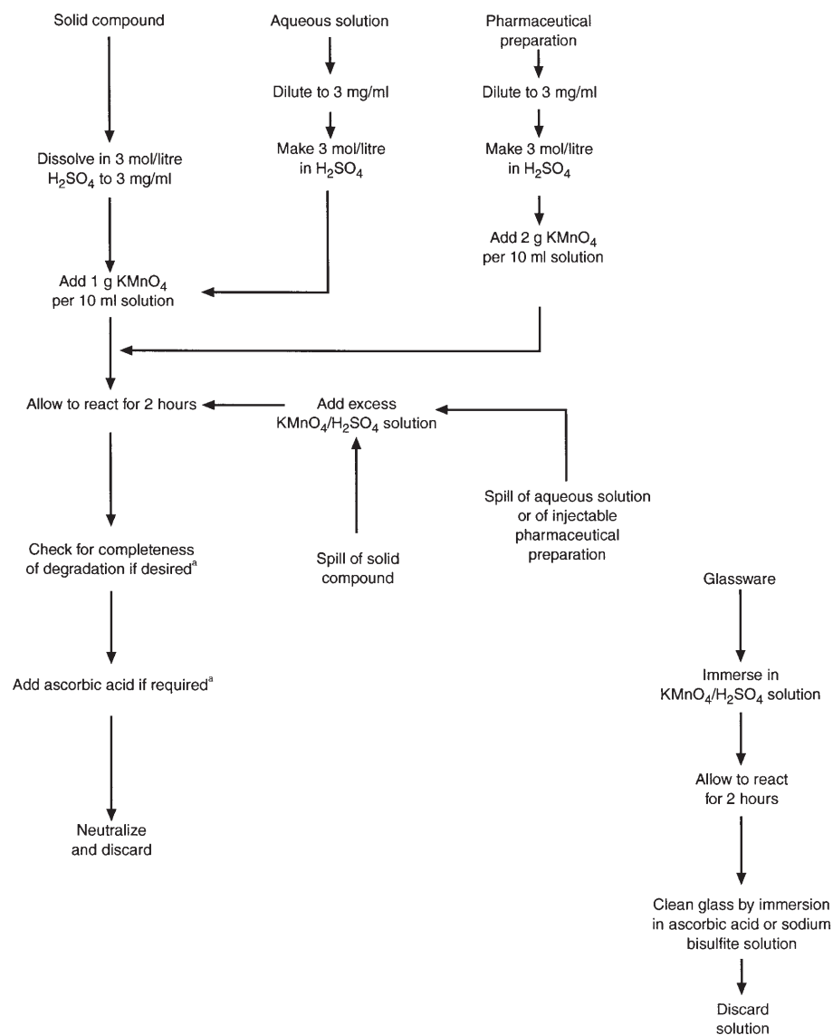
Fig. A2.1 Schematic representation of procedure for destruction of doxorubicin or daunorubicin
