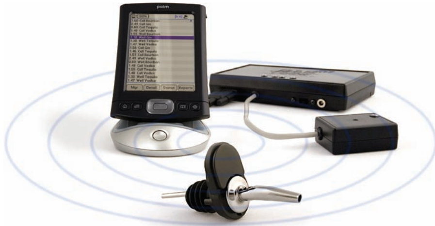
FIGURE 2.5 A wireless free-pour liquor inventory management system.
