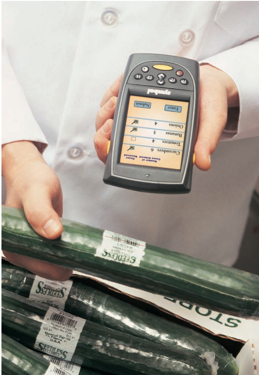
FIGURE 2.4 A bar code reader. Courtesy of Symbol Technologies, Inc.
