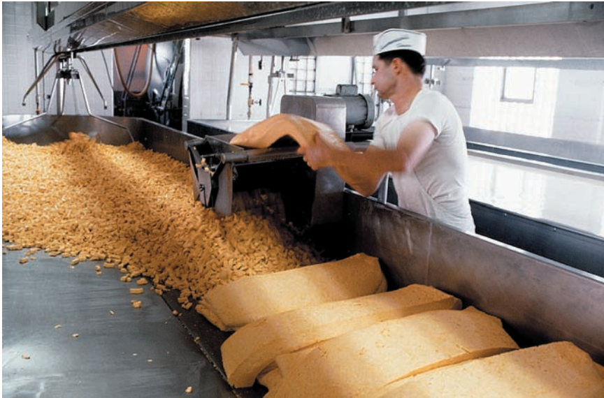
FIGURE 3.4 A cheese plant worker feeds large pieces of cheddar curd into a mill creating smaller pieces prior to pressing into the forms.
