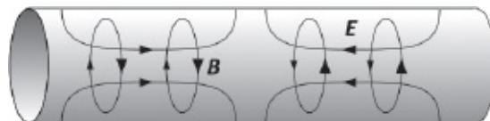
FIGURE 5.11 The wave mode excited in a cylindrical waveguide.
