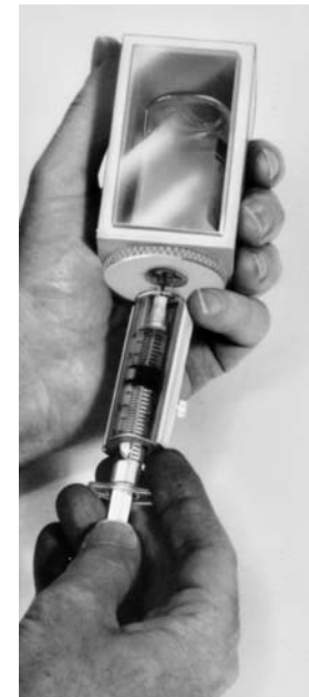
Figure 5-48. Vial shield for viewing, handling, and dispensing radioactive liquids. (Photo courtesy: Nuclear Associates, Carle Place, NY.)
