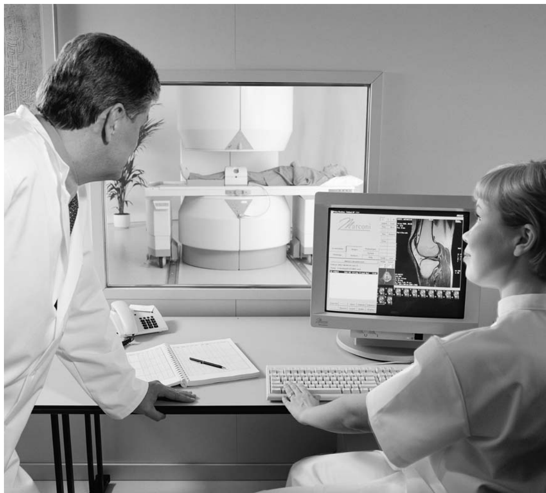
Figure 5-67. Marconi 0.23T Proview open MRI. (Illustration courtesy: Marconi Medical Systems, Cleveland, OH.)
