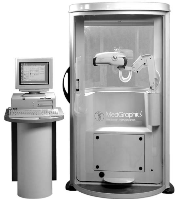
Figure 3-69. Plethysmograph for pulmonary function studies. (Photo courtesy: Medical Graphics Corporation, St. Paul, MN)
