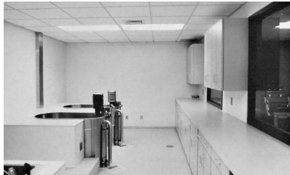
Figure 8-15. Hydrotherapy room. Note that whirlpools have been built in. (Photo courtesy: William Merc, Kessler, Merc and Associates, Chicago, IL; Photographer: Greg Merc.)
