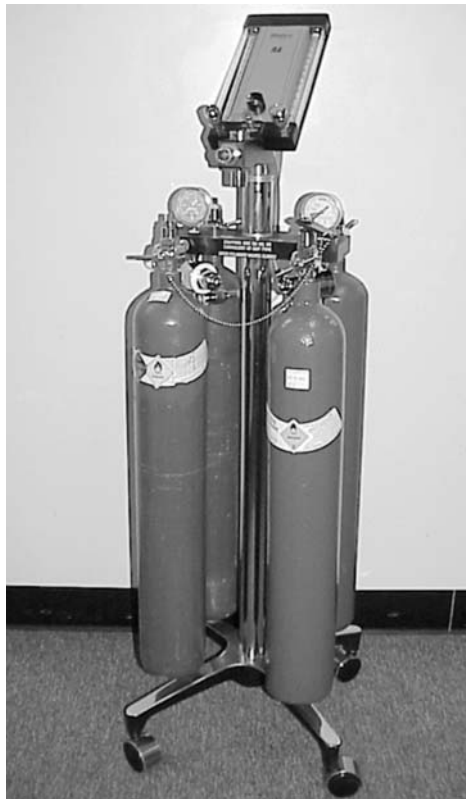
Figure 10-55. Dental analgesia flowmeter and gas cylinders on mobile stand. (Photo courtesy: Littell Industries Inc., North Hollywood, CA.)
