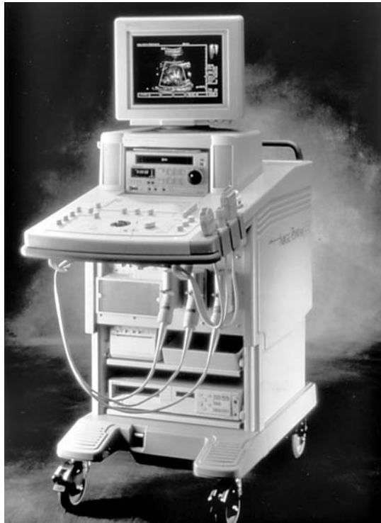
Figure 3-57. Echocardiography unit images the heart with ultrasound technology. SONOS Ultrasound Unit. (Photo courtesy: Agilent Technologies, Inc., Andover, MA.)
