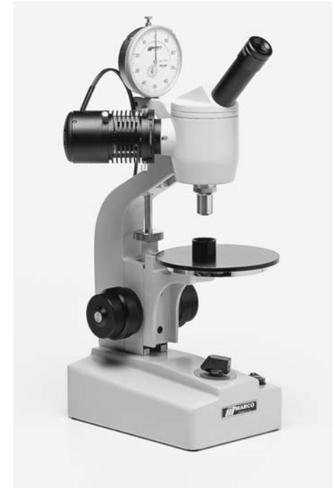
Figure 4-75. Radiusgauge™ used to measure hard or gas-permeable contact lenses. (Photo courtesy: Marco Ophthalmic, Jacksonville, FL.)
