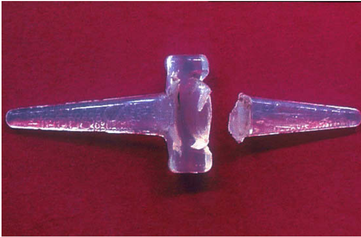
Fig A2.3. Swanson type implant where rotation is generated by elastic bending. Fracture after repeated flexure during a test. Picture provided by courtesy of Dr Tom Joyce, Centre for Biomedical Engineering, University of Durham, Great Britain.
