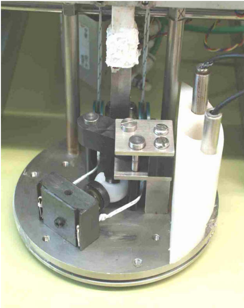
Fig A2.1. Detail view of an apparatus to test finger implants. Picture provided by courtesy of Dr Tom Joyce, Centre for Biomedical Engineering, University of Durham, Great Britain.
