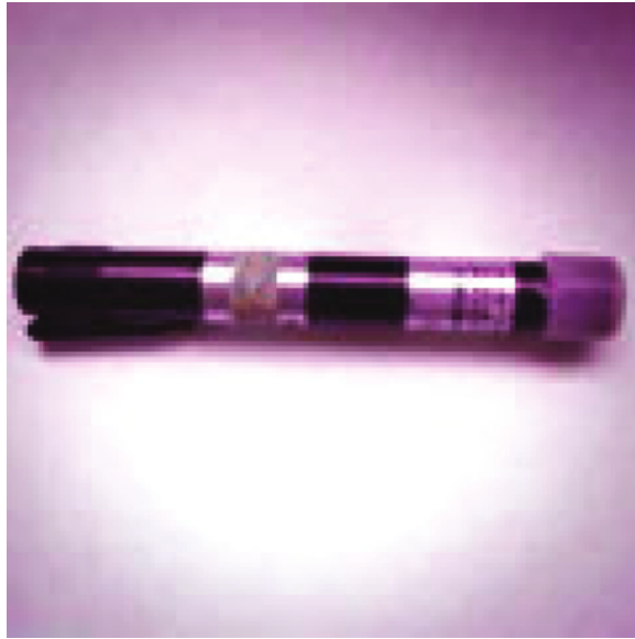
Figure 8.22 Pocket ionization chamber. (From http://www.hsa.gov.sg/html/business/crp_consultancy_instrument.html .)
