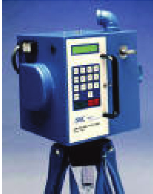
Figure 11.23 “Hi Vol” air sampler ( http://www.laurussystems.com/products/air_samplers.htm ).
