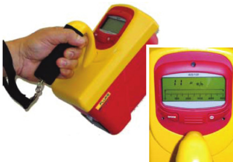
Figure 8.11 Victoreen Model 451 portable pressurized ion chamber. ( http://www.flukebiomedical.com/rms/productDataSheets/451B-ds.pdf , with kind permission from Fluke Biomedical.)
