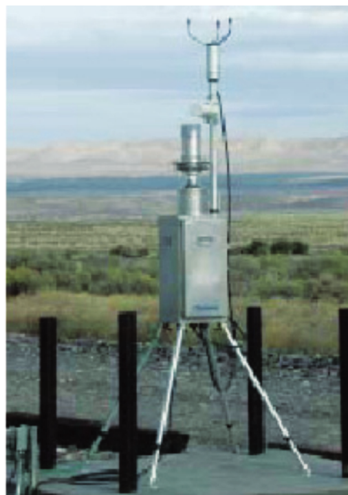
Figure 12.7 Alpha detector and continuous air monitor. (From http://www.bhi-erc.com/ .)
