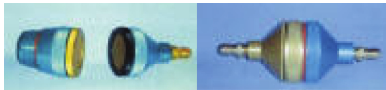
Figure 11.24 Filter holders for particulate sampling ( http://www.laurussystems.com/products/air_samplers.htm ).
