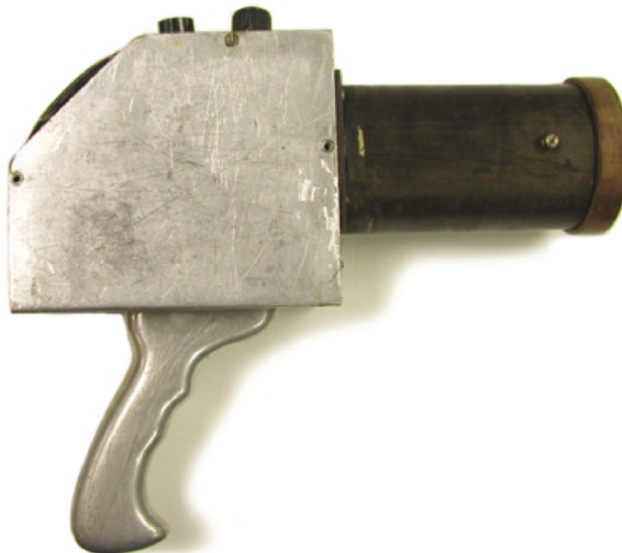
Figure 8.10 Image of an older "gun type" ionization chamber, the Hanford "Cutie Pie." (From http://www.orau.org/ptp/collection/surveymeters/hanfordcutiepie.htm .)
