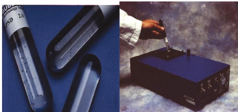
Figure 8.27 Personal bubble dosimeters (left) and dosimeter reader (right). (From http://www.bubbletech.ca .)
