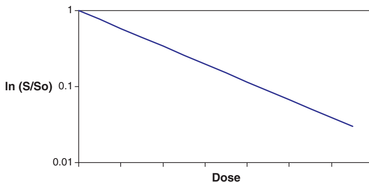
Figure 6.14 Cell survival curve: high LET radiation, single exponential.
