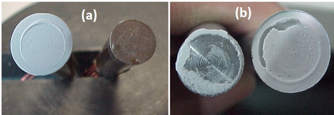
Fig. 4. Adhesion tests; (a) before and (b) after being delaminated from the metallic substrate.
