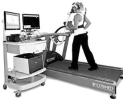
FIGURE 15 VO_{2\text{max}} measurement through a modern metabolic cart during a graded exercise test on a treadmill (Stress test).
