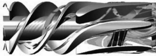
FIGURE 17 CFD flow analysis of bearing design for DeBakey VAD (23).
