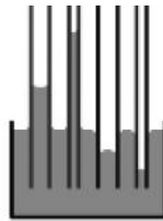
Left two capillaries = contact angle less than 90°; Right two capillaries = contact angle greater than 90°.
