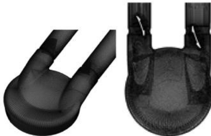
FIGURE 14 CFD flow analysis for Artificial Heart: De Bakey VAD (23).
