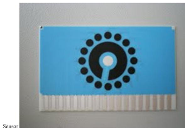
Fig. 23 Screen-printed array of 16 electrodes, suitable for modification of each surface and obtaining a BioET, materials available from Dropsens S.L., http://www.dropsens.com , Oviedo, Spain
