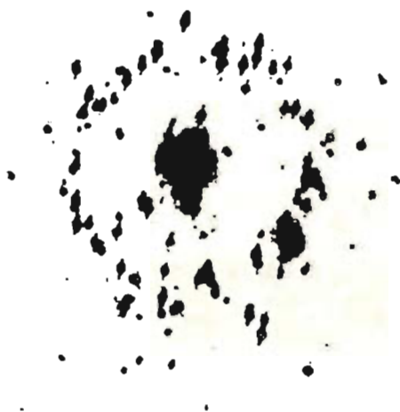
Fig. 3.3. Cerenkov cone for detected photons and ionization products in a gas filled detector for \sim 10 individual particle passages. (From Ref. B.1 and Ref. B.2, with permission.)
