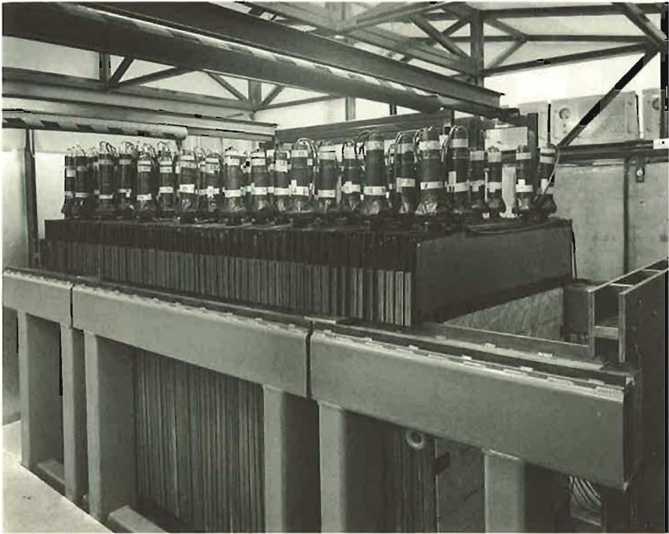
Fig. 11.6. Photograph of a sampling calorimeter showing interspersed lead and scintillator (EM) and iron and scintillator (HAD) planes. (Photo – Fermilab.)
