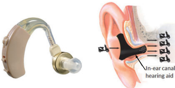
Fig. 12.26: In-ear canal hearing aid. External sound is amplified by the hearing aid and the drum head is exposed to an increased pressure amplitude.
