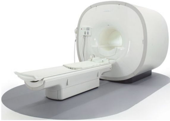
Fig. 15.32: Clinical 1.5 T MRI system with an RF power of 1 kW, field gradient of 33 mT/m, FOV of 53 cm, and a power consumption during scanning of 22 kW. Vendor: Philips, The Netherlands.
