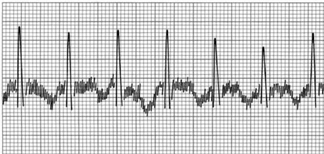
FIGURE 4–7 • 60-cycle interference. 60-cycle interference can be caused by ungrounded electrical equipment in the room.
