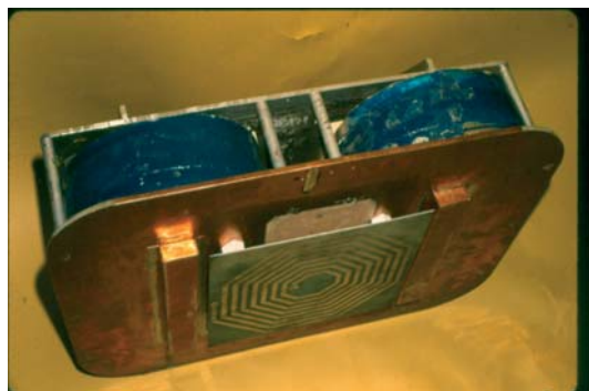
Figure 2.1. A single-sided NMR magnet and coil built by Southwest Research Institute showing the “pancake” coil in the center and the electromagnet driven by the blue coils. (Photo supplied by Armando De Los Santos, Southwest Research Institute.)
