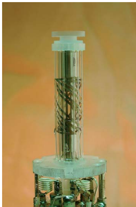
Figure 22.9. A triple-resonance ( ^1\text{H}/^{13}\text{C}/^{15}\text{N} ) PFG high-resolution liquid probe with a low- \mu millipede coil.
