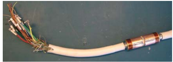
Figure 25.12. Floating shield cable trap installed on a system cable.
