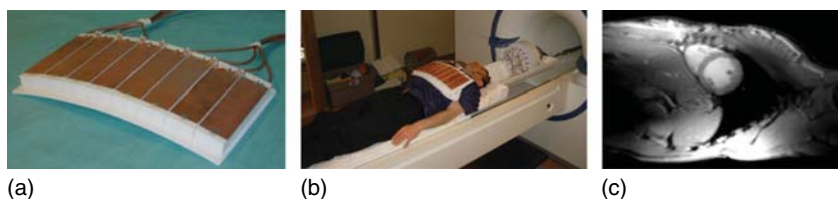
Figure 13.5. Multichannel transceiver surface coils. (a) One of a pair of eight channel transmission line (TEM) arrays. With one coil atop and the other below the subject’s torso (b), cardiac images are acquired (c).
