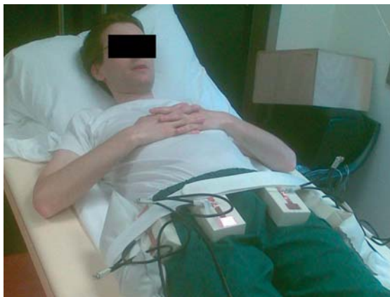
Figure 17.11. Array of radiative antennas around pelvis for volunteer measurement.
