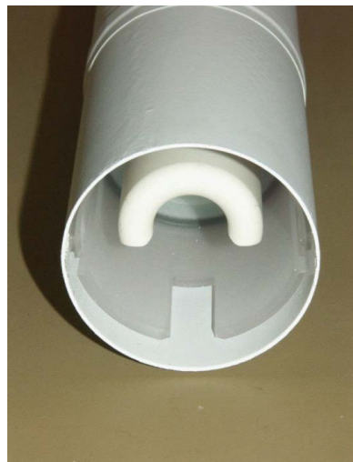
Figure 20.4. Principle design of a cryo-coil Dewar and cryostat: (1) RF coil; (2) cold finger; (3) ceramic Dewar; and (4) heater.
