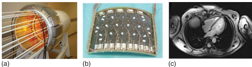
Figure 13.6. Body coil (a) with half of receiver pair (b) used to acquire image (c) with 16 channels transmitting and 32 channels receiving.
