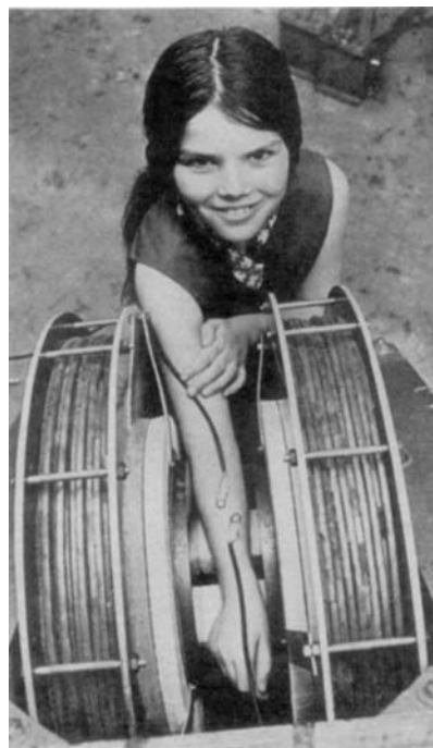
Figure 1.1. A copy of Figure 1.1 from the 1970 Science magazine article by O. C. Morse and J. R. Singer titled “Blood Velocity Measurements in Intact Subjects”. 3 This figure shows a volunteer with her arm in the space between the pole faces of a 0.36 T (15.4 MHz) iron magnet. Two surface coils separated by 2.5 cm are visible, lying over a vein on top of the subject’s forearm. The upstream coil served to perturb the flowing venous blood ^1\text{H} (water) magnetization via adiabatic fast passage. The downstream surface coil served to detect ^1\text{H} the magnetization as a function of time following upstream perturbation. This time-of-flight “angiography” demonstration is the earliest known (to this author) published use of surface coils in vivo . (Reproduced from Ref. 3. © American Association for the Advancement of Science, 1970.)
