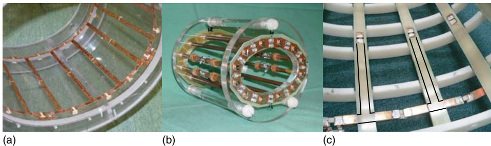
Figure 11.7. Typical construction methods utilizing (a) copper strips and chip capacitors, (b) copper rods for the legs and circuit board end-rings, and (c) copper bars and capacitors with ribbon leads.
