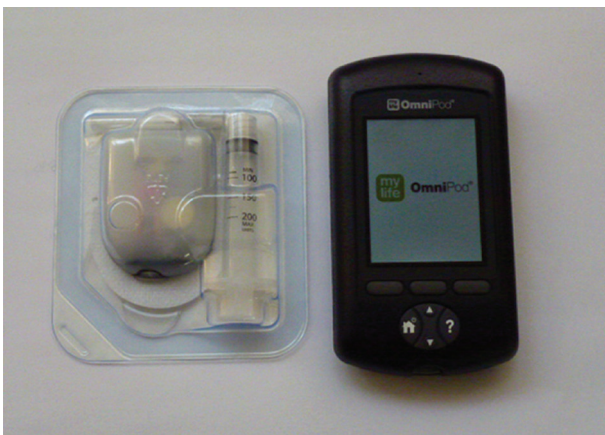
Figure 31.4 A 'patch' pump (OmniPod Insulin Management System, Ypsomed). On the left is the single-use pump, usually applied to the abdomen, and which is discarded and a new one applied once the single-fill insulin reservoir containing 200 units is finished (about 2–4 days). Right: the separate remote control device for the pump with an integrated blood glucose meter.
