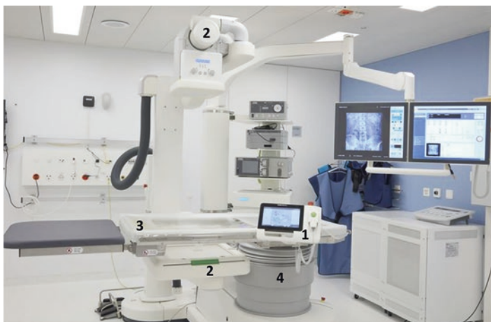
FIGURE 1.1 Urological multifunctional table with SWL generator. (1) Operating unit, (2) X-ray, (3) Examination table, (4) Shock wave generator
