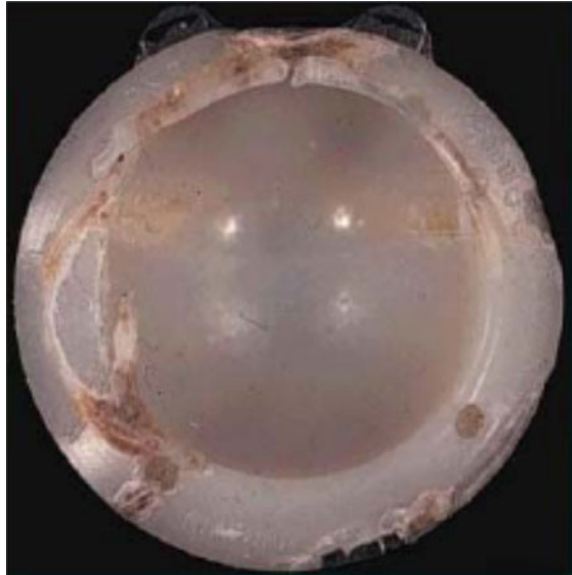
Fig. 7.6 Example of worn UHMWPE acetabular cup for total hip replacement [45]
