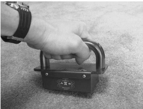
**FIGURE 30-7** A handheld magnet of at least 100 mT strength can be used to screen objects before taking them into the magnetic resonance imaging room. (Courtesy Emanuel Kanal, Pittsburgh, PA.)
