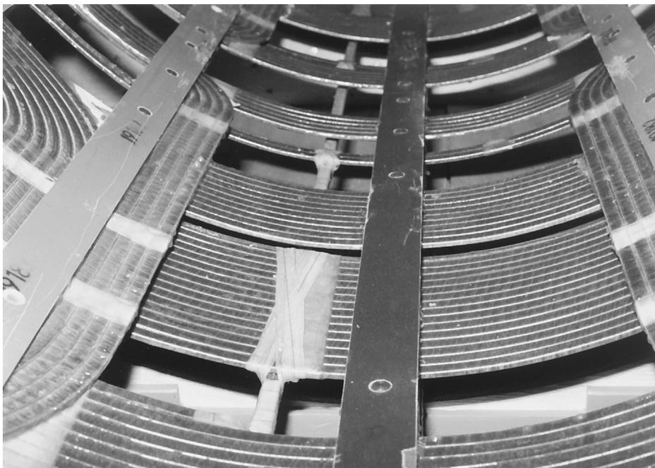
**FIGURE 11-3** Gradient coils consist of large, band-type conductors.
