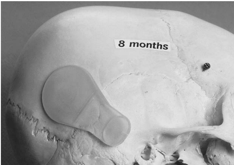
FIGURE 8.27. Photograph of the Nucleus CI 24 receiver-stimulator placed over the flatter section of the skull of an 8-month-old infant.
