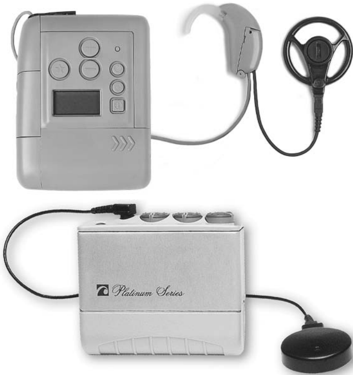
FIGURE 8.18. Top: The Cochlear Limited Nucleus 24 body-worn SPrint for the regular and research speech-processing strategies (Reprinted with permission from Cochlear Limited). Bottom: The Clarion Platinum body-worn speech processor (Reprinted with permission from Advanced Bionics Corporation).
