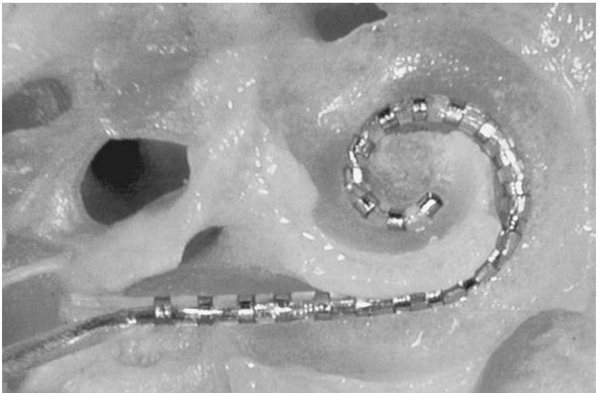
FIGURE 8.39. Human temporal bone insertion with the precurved array and the bone uncapped to expose it lying in the scala tympani. (Reprinted from the Cooperative Research Centre for Cochlear Implant Speech and Hearing Research Annual Report 1994–95, with permission.)
