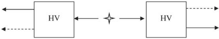
Figure 8.6 In some circumstances atoms can be made to emit a pair of photons in rapid succession. The two members of each pair move away from the source in different directions. In the set-up shown, the light source is in the centre; the right-hand apparatus measures the HV polarization of one of the two photons while that of the other is measured on the left. Whenever a right-hand photon is recorded as horizontally polarized that on the left is found to be vertical and vice versa.
