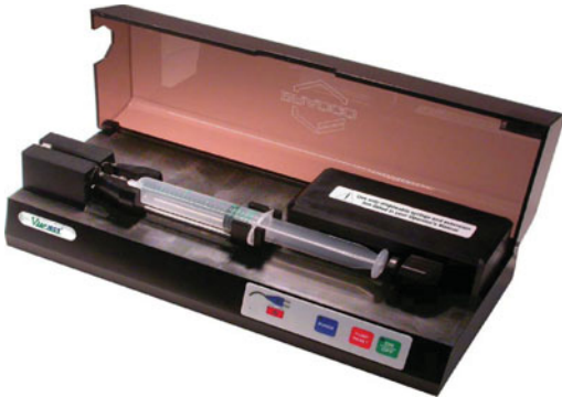
Fig. 9.5 SonoVue ® pump Image courtesy of Bracco International BV. The pump provides continuous rotation of the syringe in order to prevent accumulation of the microbubbles in the upper parts of the syringe.
