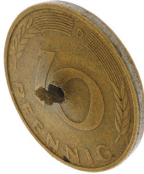
Fig. 2.3 Photograph of a ten-penny coin of the former Federal Republic of Germany, perforated by a high-speed water drop at the High Speed Physics Laboratory of the Saarland University, Saarbrücken, Germany. The experimental arrangement was used to show that a single water drop can produce severe damage to solid structures if accelerated at supersonic speed. (Courtesy of E. Häusler)
