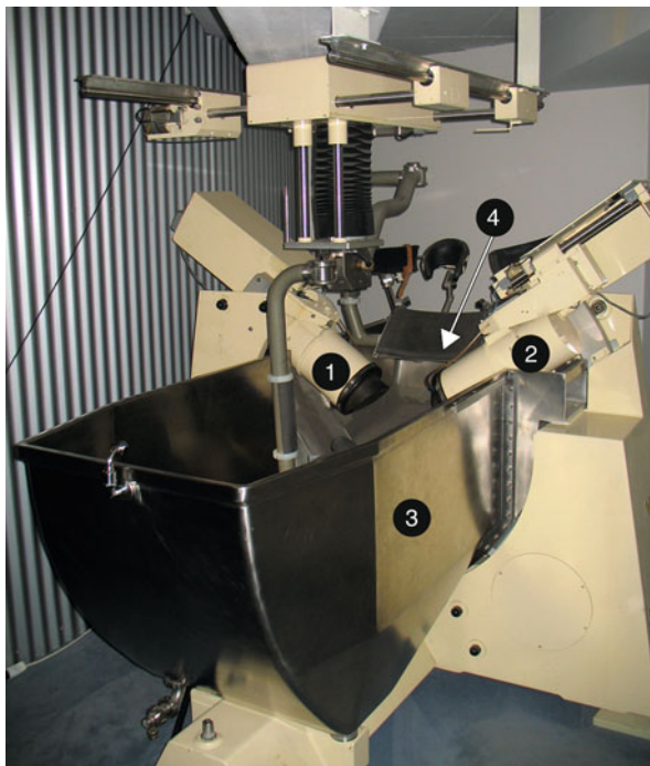
Fig. 2.5 Photograph of the Human Model 1 (HMI) lithotripter (Dornier MedTech GmbH, Wessling, Germany), used to perform the first extracorporeal shock wave lithotripsy in 1980, showing (1) the right (as seen from the patient) and (2) the left image intensifier of the biplanar fluoroscopy system, (3) the water tub, and (4) the patient stretcher. The lithotripter was donated to the German Museum (“Deutsches Museum”) in Bonn, Germany. (Courtesy of C. Chaussy)
