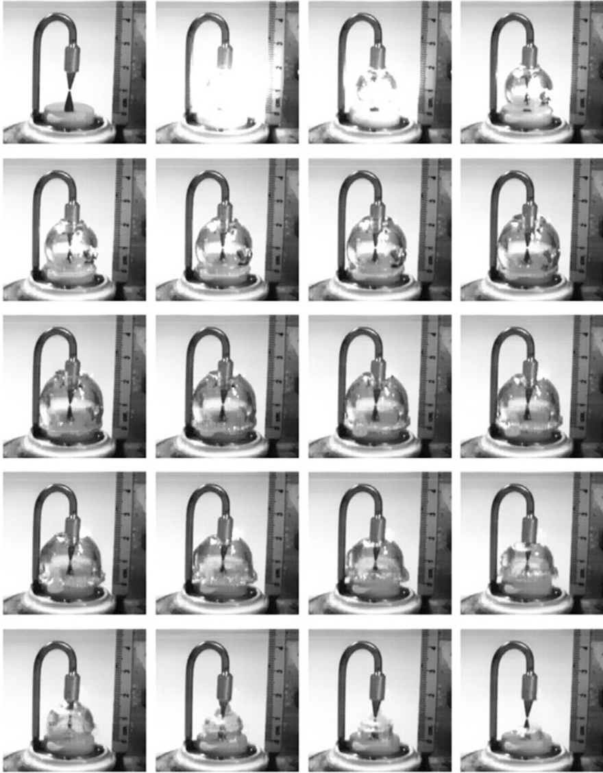
Fig. 5.14 High-speed photographic sequence ( 156.8 \mu\text{s} between images) of an underwater electric discharge between two electrodes (capacitance 80 \text{ nF} , voltage 16 \text{ kV} ). The sequence starts at the upper left corner and continues from left to right until it ends at the lower right corner. (Photograph: E. Fernández)
