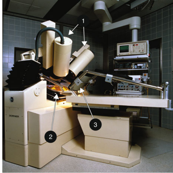
Fig. 2.10 Photograph of the Human Model 4 (HM4) extracorporeal shock wave lithotripter, showing (1) the image intensifiers of the biplanar X-ray system, (2) the water cushion, and (3) the patient stretcher. (Courtesy of Dornier MedTech GmbH, Wessling, Germany)
