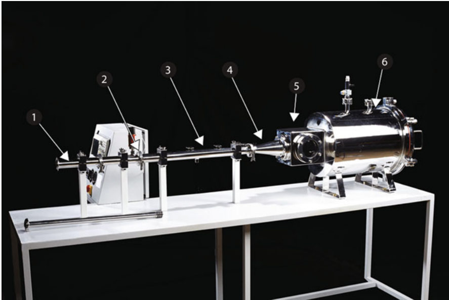
Fig. 7.3 Photograph of a hand driven shock tube used as a teaching tool, showing (1) the driver section, (2) the diaphragm station, (3) the driven section, (4) the convergent–divergent nozzle, (5) the test section, and (6) the dump tank. (Courtesy of KPJ Reddy)
