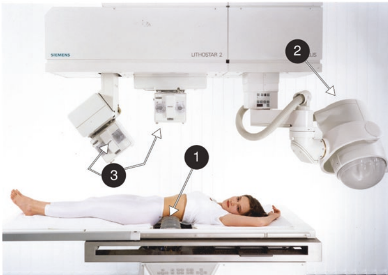
Fig. 5.43 Photograph of the Lithostar 2 Plus lithotripter with three electromagnetic shock wave sources, showing (1) the left undertable shock wave source, (2) the overhead shock wave source with in-line ultrasound scanner, and (3) the X-ray sources. (Courtesy of Siemens Healthcare GmbH, Erlangen, Germany)
