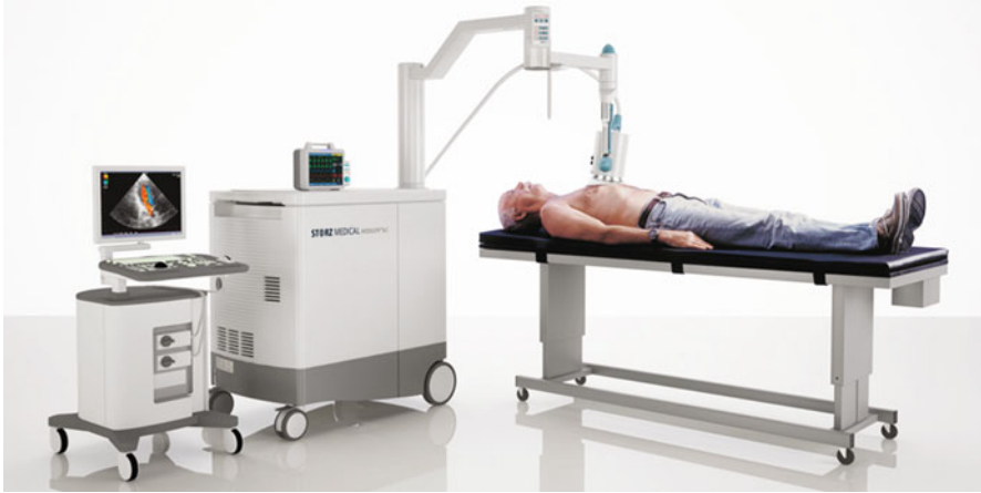
Fig. 6.21 Photograph of the Modulith SLC electromagnetic shock wave source (Storz Medical AG, Tägerwil, Switzerland) with in-line ultrasound localization, designed for noninvasive cardiac revascularization
