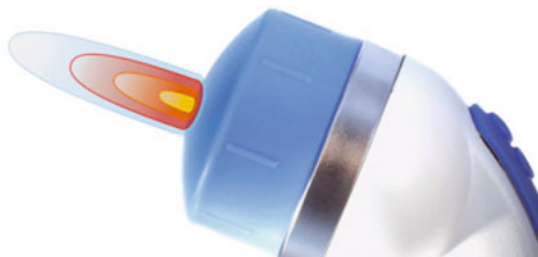
Fig. 6.6 Image of the Aries shock wave source showing the geometry of different isobars of the focal zone. The penetration depth can be varied by modifying the energy settings. As the energy rises, the 5 MPa isobar intersects the beam axis at a larger distance from the therapy head. (Courtesy of Dornier MedTech GmbH, Wessling, Germany)
