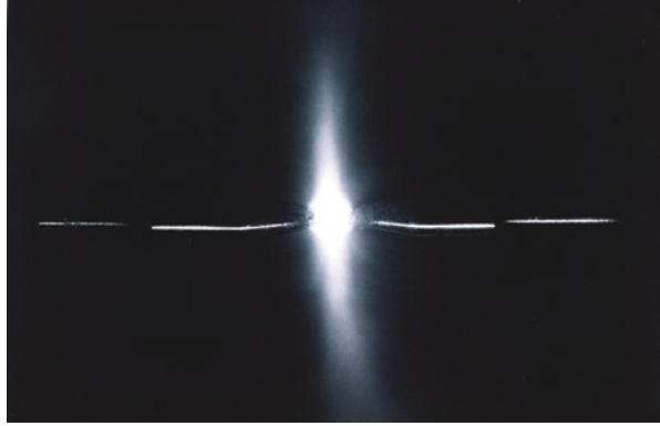
Fig. 5.12 Photograph of a high-voltage discharge between two electrodes immersed in water. (Photograph: A. Sánchez)
