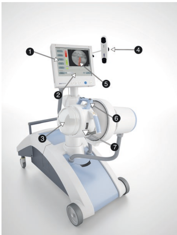
Fig. 5.20 Photograph of the basic version of the LithoSpace in its undertable position, showing (1) the touch panel, (2) the coupling pressure indicator, (3) the water cushion, (4) the stereo camera, (5) a superimposed therapeutic volume on the X-ray image, (6) the reflector panel, and (7) the shock wave source. (Courtesy of Jena Med Tech GmbH, Jena, Germany)
