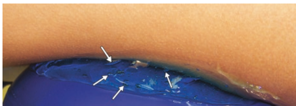
Fig. 5.71 Bad shock wave coupling through a water cushion and a bubbly ultrasound gel. The arrows point at a few air bubbles
