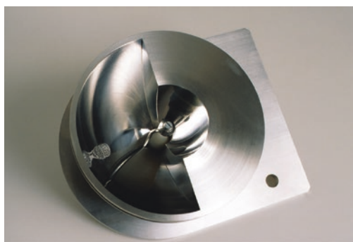
Fig. 5.32 (a) Schematic and (b) photograph of a research stainless steel bifocal reflector, designed to fit on a Tripter Compact (Direx Systems Corporation, Canton MA, USA) electrohydraulic lithotripter
