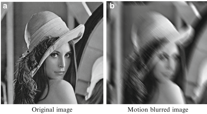
Fig. P5.6 Motion blurred 512 \times 512 image with a = b = 0.2 and C = 1
