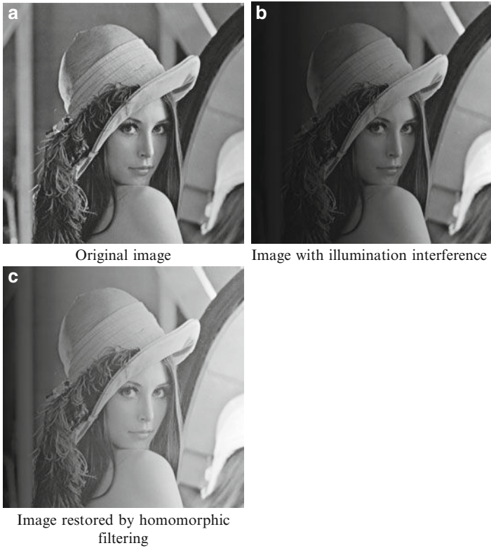
Fig. 5.20 Homomorphic filtering of an image with illumination interference
