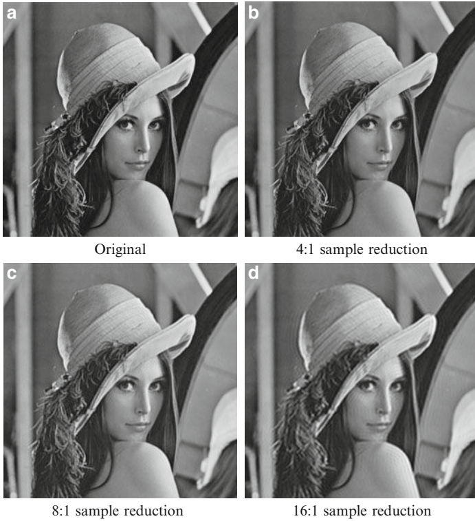
Fig. 5.37 Basis restriction zonal filtered images in the DCT domain (geometrical zonal sampling – see Fig. 5.35)
