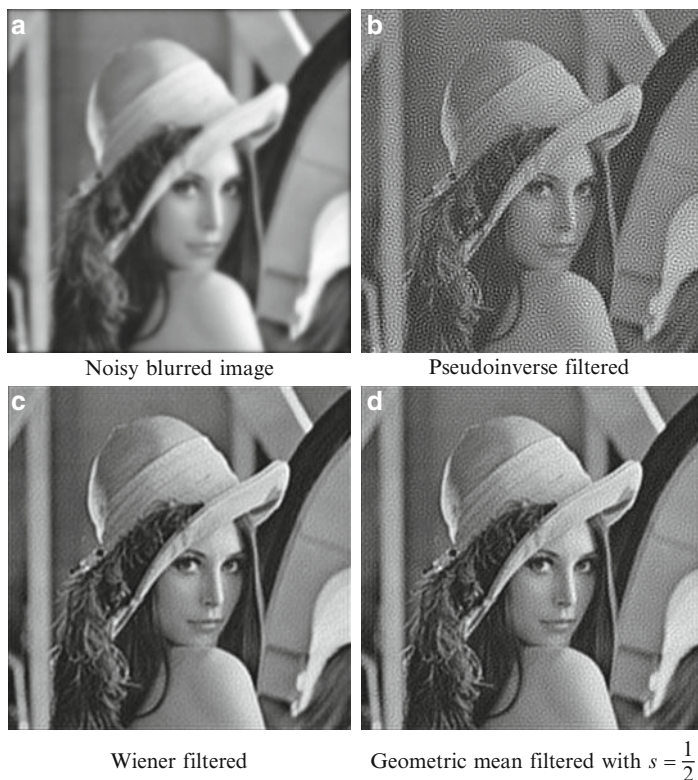
Fig. 5.27 Geometric mean filtering
