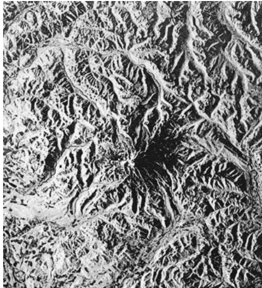
FIGURE 33.2 SAR image of Mt. Rainier in Washington State taken from shuttle imaging radar.
