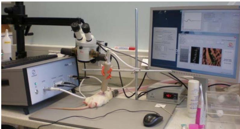
Figure 20.10 Transient micro-elastography using FibroScan® LAB for measurements in small laboratory animals. Source: courtesy of Pr Sebastian Mueller, setup at the University of Heidelberg.
