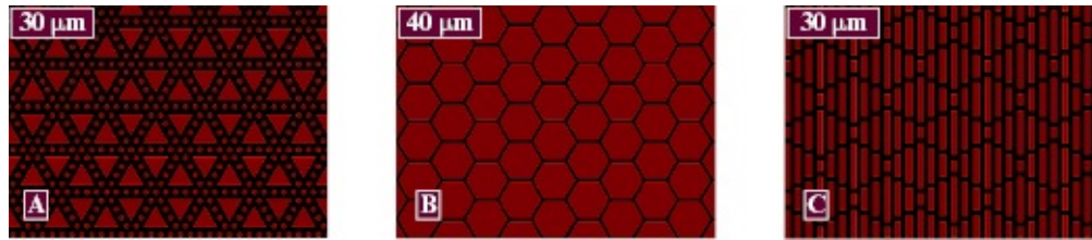
Figure 5.5 Designed patterns drawn in AutoCAD ® . (A) 10- \mu\text{m} equilateral triangles surrounded by 2- \mu\text{m} (diameter) circles spaced by 2 \mu\text{m} . (B) 20- \mu\text{m} height hexagons spaced by 2 \mu\text{m} . (C) Sharklet AF ™ design composed of 2- \mu\text{m} wide ribs of varying lengths including 4, 8, 12, and 16 \mu\text{m} . Ribs are spaced by 2 \mu\text{m} in all directions.
