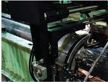
Figure 5-84 Phased array inspection of coiled tube seam weld: principle ( top ) and industrial system ( bottom ).
