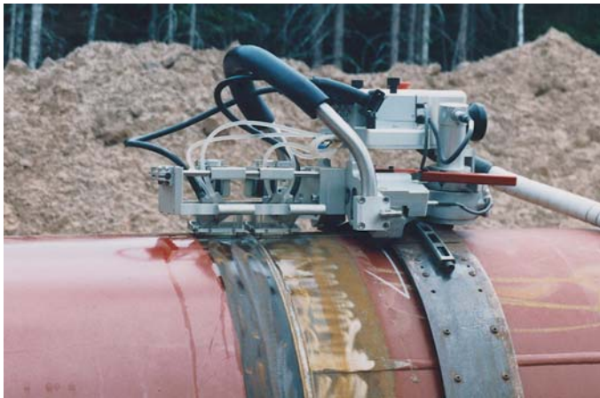
Figure 5-61 Pipeline welding band and probe pan. This pan contains two well-protected linear phased array probes and can significantly outperform competing multiprobe technologies.
