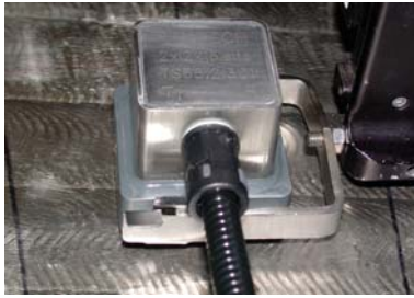
Figure 5-38 Waterproof TRL phased array probes for pressure vessel nozzle.
