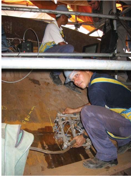
Figure 5-63 Hand scanner for weld inspections. This version contains either phased arrays or multiple conventional transducers (see "Rapid Detection TECHnique" in section 4.2.10, p. 186, and "PV-100" in section 5.7.2, p. 233).
