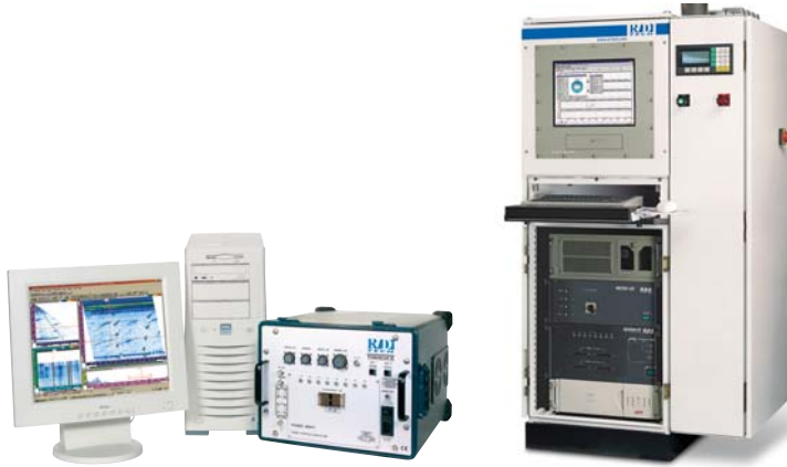
Figure 5-6 R/D Tech Tomoscan III PA ( left ) and QuickScan PA ( right ). These show the instruments in a typical configuration and installation.
