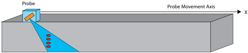
Figure 4-2 Linear scan pattern for probe characterization.
