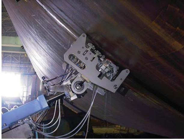
Figure 5-60 Example of rotating vessel for phased array inspection of pressure vessels under construction using a fixed head containing two linear arrays with linear and electronic scanning.
