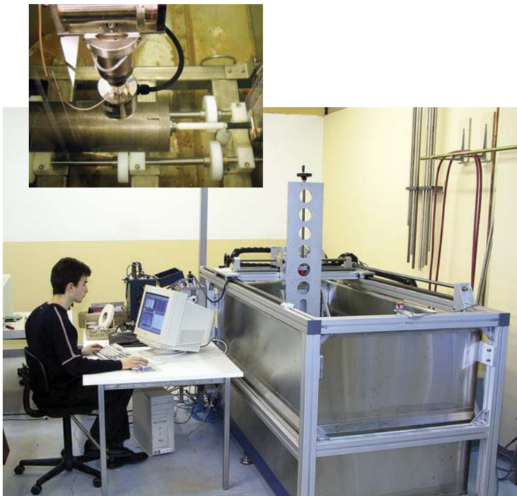
Figure 5-14 Immersion testing with a rho-theta probe on titanium billets.
