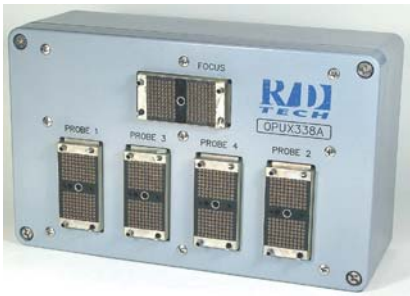
Figure 3-59 4:1 breakout box used with multihead inspection.
