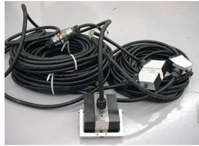
Figure 5-38 Waterproof TRL phased array probes for pressure vessel nozzle.
