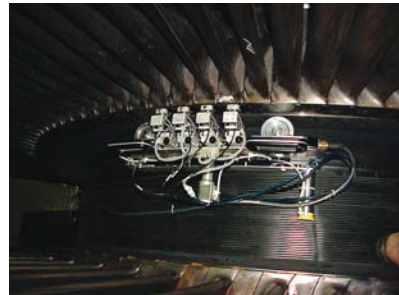
Figure 3-59 4:1 breakout box used with multihead inspection.
