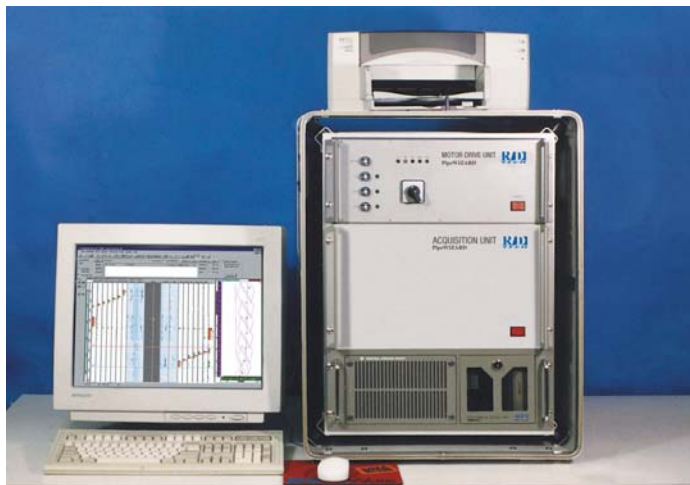
Figure 5-70 PipeWIZARD phased array system showing instrumentation box (computer, Tomoscan FOCUS, driver box), 21-in. monitor, and keyboard.
