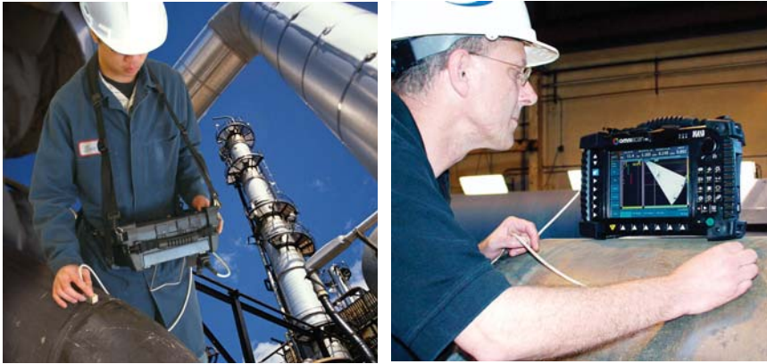
Figure 5-83 Inspection of pipe welds in a refinery with an OmniScan: on site ( left ); OmniScan with S-scan display ( right ).
