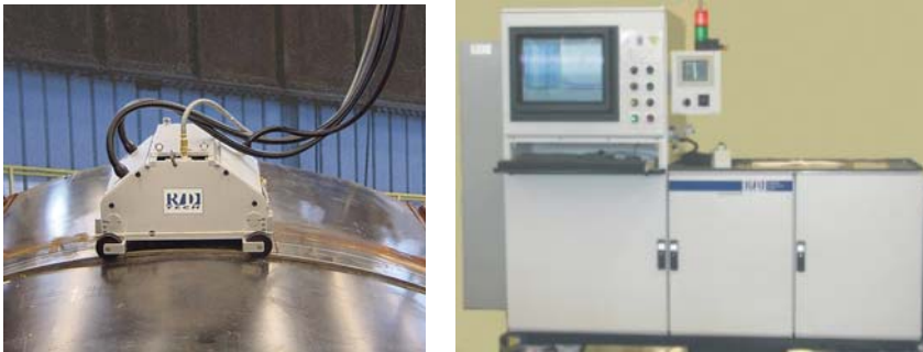
Figure 5-59 Photos of PV-300 probe pan ( left ), and cabinet containing three Tomoscan FOCUS or Tomoscan III systems, EC array instrumentation, and coupling system ( right ).
