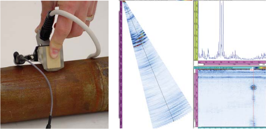
Figure 5-40 Phased array detection of fatigue cracks in CANDU ® feeder tubes: scanning setup ( left ) and crack detection ( right ).
