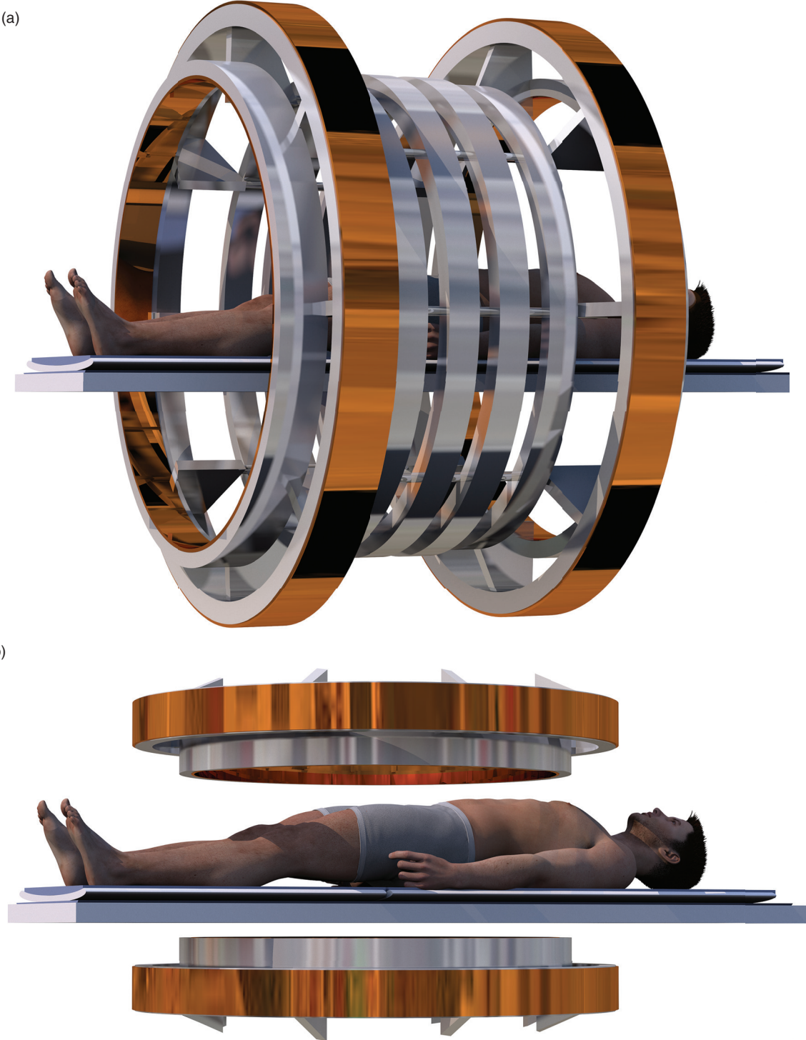
Figure 9.5 Differences in solenoid configuration in (a) closed-bore and (b) open MRI scanners.
