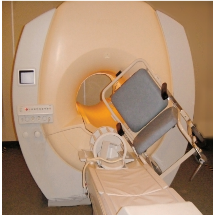
Figure 10.4 Ferromagnetic wheelchair taken into an actively shielded magnet room. No attraction was appreciated until the chair was moved close to the end of the bore.
