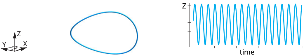
Figure 5.24: For slightly higher values of b_1 , the system exhibits a stable oscillation.
