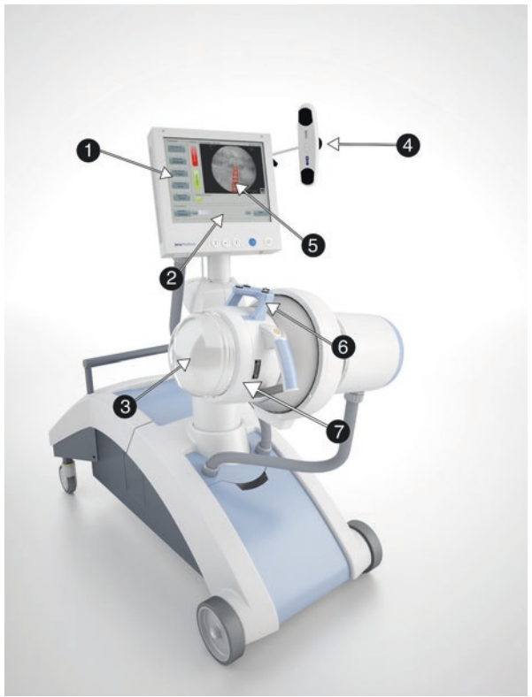
Fig. 5.20 Photograph of the basic version of the LithoSpace in its undertable position, showing (1) the touch panel, (2) the coupling pressure indicator, (3) the water cushion, (4) the stereo camera, (5) a superimposed therapeutic volume on the X-ray image, (6) the reflector panel, and (7) the shock wave source. (Courtesy of Jena Med Tech GmbH, Jena, Germany)
