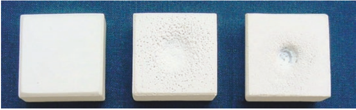
Fig. 4.5 Photograph of three (30×30×14.3 mm) AST 110 stone models (High Medical Technologies, Kreuzlingen, Switzerland), before ( left ) and after exposure to 500 underwater shock waves generated with an electrohydraulic ( center ) and a piezoelectric ( right ) shock wave source
