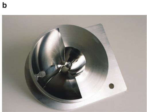
Fig. 5.32 (a) Schematic and (b) photograph of a research stainless steel bifocal reflector, designed to fit on a Tripter Compact (Direx Systems Corporation, Canton MA, USA) electrohydraulic lithotripter
