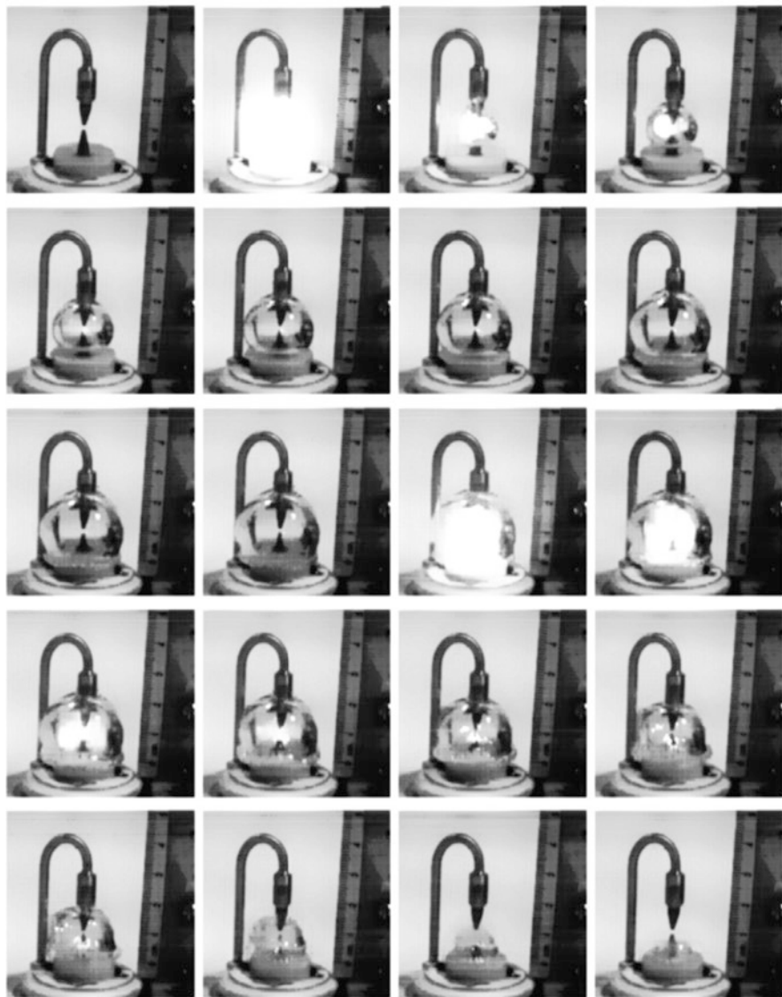
Fig. 5.29 High-speed photographic sequence ( 160.5 \mu\text{s} between images) of two underwater electric discharges between two electrodes, generated at a delay of 1.56 \text{ ms} (capacitance 160 \text{ nF} , voltage 16 \text{ kV} ). The sequence starts at the upper left corner and continues from left to right until it ends at the lower right corner. The first electric discharge occurred shortly before the second image and the second discharge occurred between the 10th and the 11th image. (Photograph: E. Fernández)
