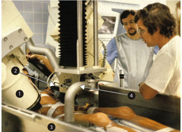
Fig. 2.6 Christian Chaussy ( right ) supervising patient positioning for SWL with the Dornier HMI extracorporeal shock wave lithotripter. The photograph shows the two image intensifiers (1) and (2) of the biplanar fluoroscopy system, the stainless steel water tub (3) and the support of the patient stretcher (4). (Courtesy of C. Chaussy)
