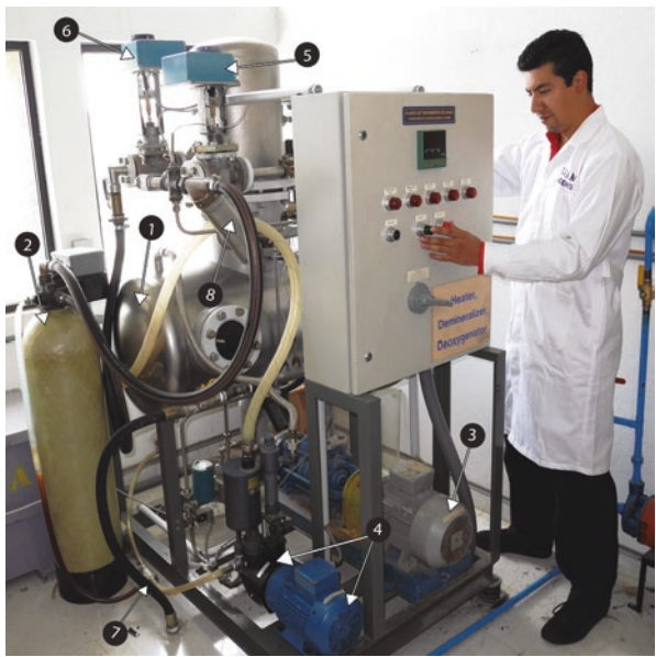
Fig. 5.17 Photograph of the water treatment plant (Wiegand GmbH, Ettlingen, Germany) used to deionize and degas the water of an HM3 lithotripter (Dornier MedTech GmbH, Wessling, Germany), showing (1) the degasser tank, (2) the deionization tank, (3) the degasser motor that pumps water to the tub, (4) the vacuum motor and the pump that creates vacuum in the degasser tank, (5) the mixing valve, (6) the input valve to the degasser tank, (7) the output to the tub, and (8) the water filter. (Photograph: F. Fernández)
