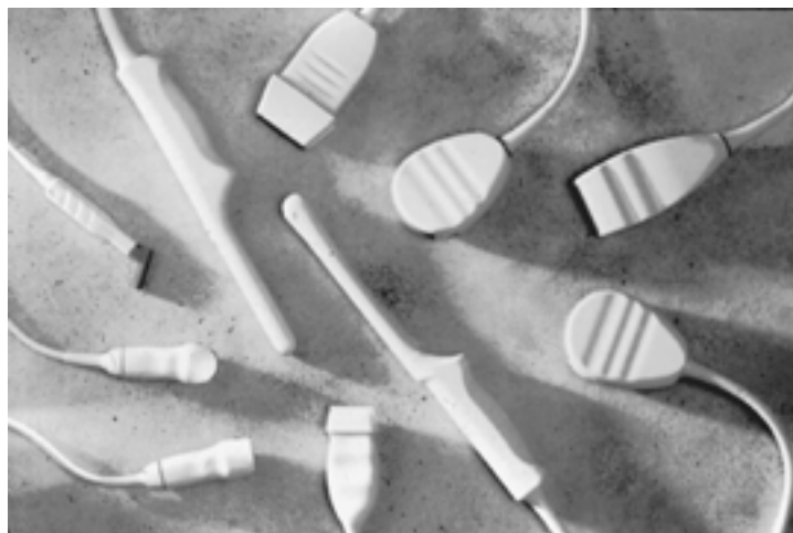
FIGURE 13.1 Representative ultrasonic scan heads (array transducers). Clockwise from top: linear array, curvilinear abdominal array, high frequency linear, another curved abdominal, curved intravaginal, two phased arrays, highly curved array, side-looking linear array for intraoperative use, and microcurved intravaginal array. (Courtesy of ATL Ultrasound.)
