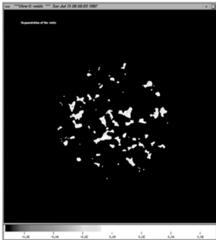
FIGURE 15.19 Segmentation results of the air, including cracks and voids, within the asphalt sample for the slice plane shown in Figure 15.16 .
