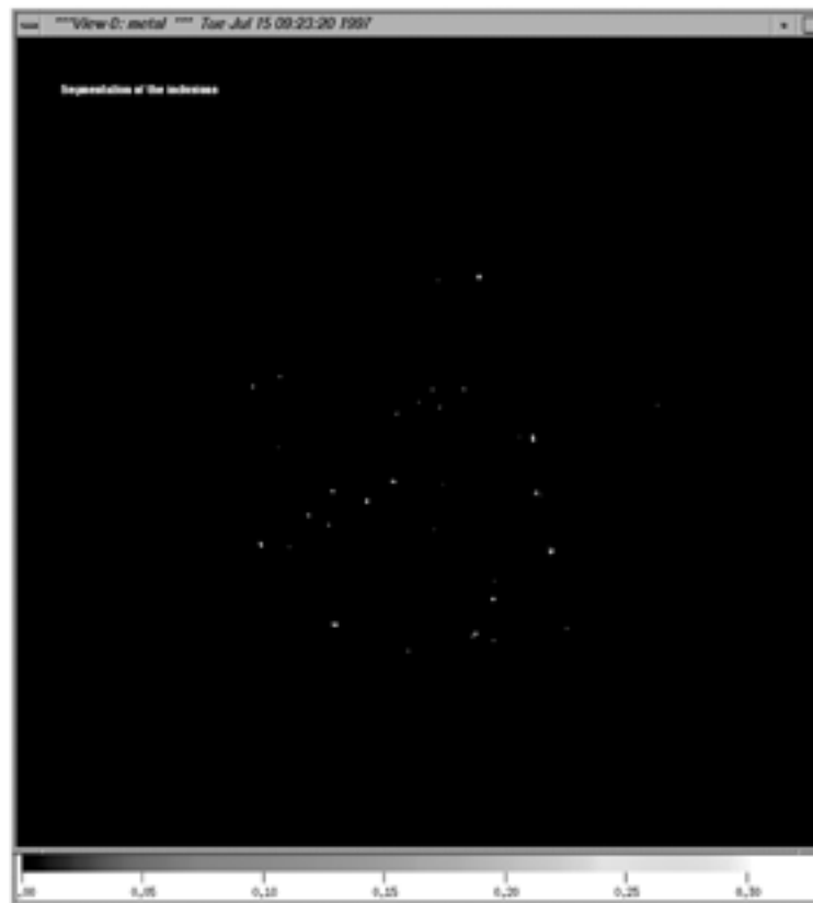
FIGURE 15.20 Segmentation results of apparent metal or high atomic number inclusions within the asphalt sample for the slice plane shown in Figure 15.16 .
