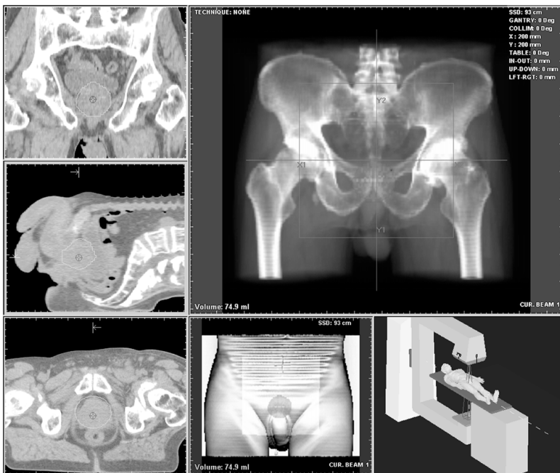
FIGURE 20.11 Another screen configuration of EXOMIO. In addition to the view windows shown in Figure 20.10 , a coronal and sagittal reconstructed image window are included. The delineated GTV/CTV is shown on different CT images, BEV, and 3D surface rendering window.
