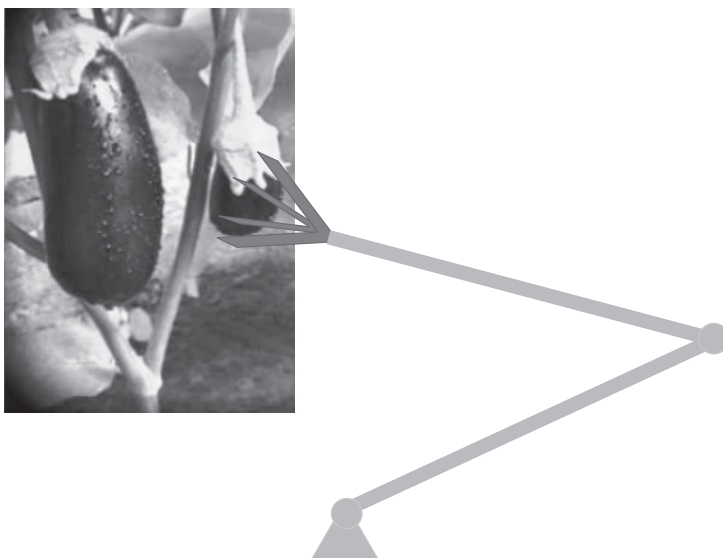
Fig. 2. A 2-DOF vegetable gripper.
