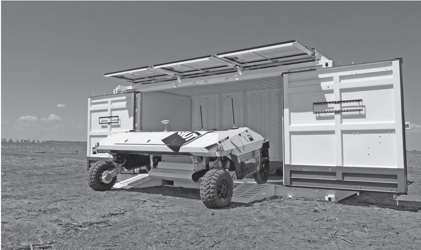
Fig. 1. Robotic system for weed and crop management. AgBotII robotic platform with underhanging weeding implement and replenishment pod.
