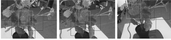
Fig. 11. Leaf tracking on several frames. Yellow bounding box indicates the target leaf that is being tracked; blue boxes indicate other detections in the frame; keypoints are highlighted on the leaves.
