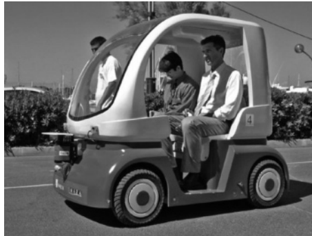
Fig. 1.37. The Cycab is an electrically-driven vehicle for autonomous transportation in urban environments (courtesy of INRIA)
