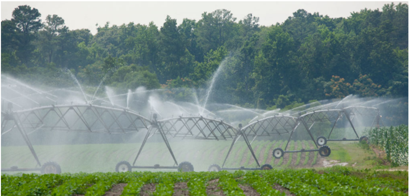
Fig. 12.5 Impact sprinklers on top of pivot
