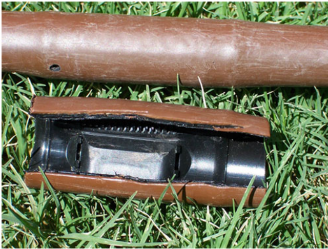
Fig. 15.6 Inline drip tubing
