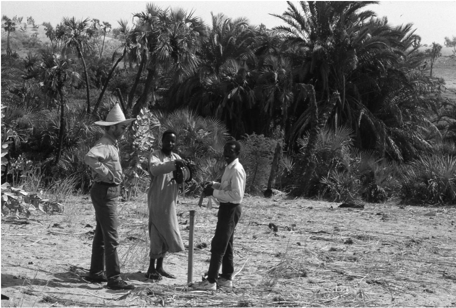
Figure 5.8 Monitoring the depth to the water table with a piezometer to assess rates of recharge and sustainable abstraction at an oasis in the Manga Grasslands in north-east Nigeria (MKVC).
