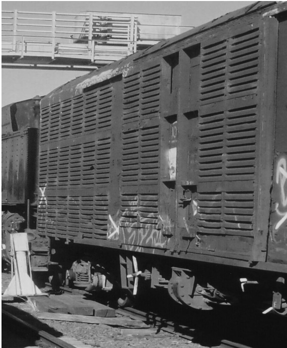
FIGURE 8.3 One type of louvered rail vans that was used for long distance transport of bananas in Australia.
