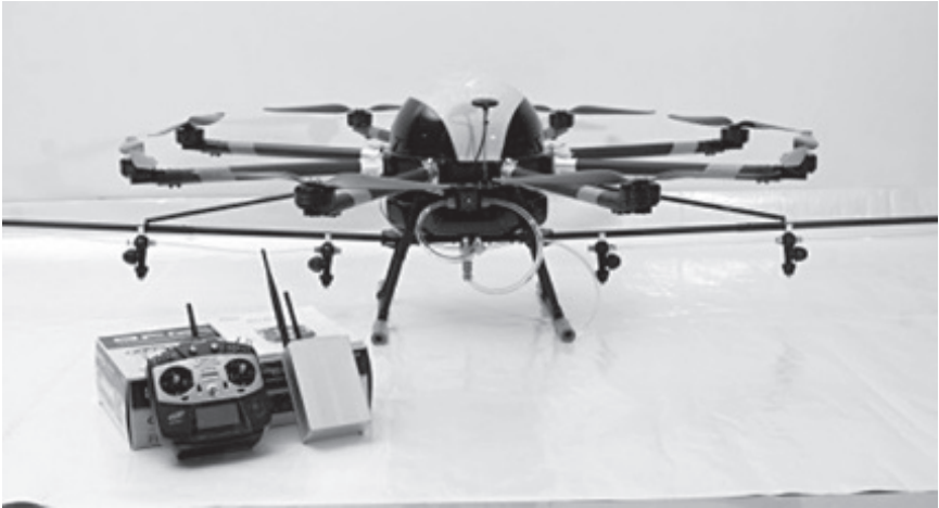
PLATE 7.4 Vero 8A—A sprayer drone used in Agricultural fields.
