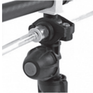
PLATE 7.3 A spray nozzle and accessories attached to drones to spray pesticides.
