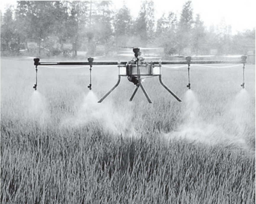
PLATE 7.5 An agricultural drone spraying pesticides on to a rice crop.
