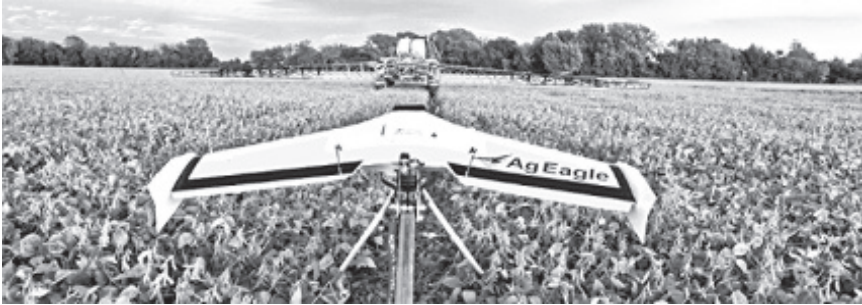
PLATE 4.8 A flat-winged drone being readied to take off and scout the soybean field.
