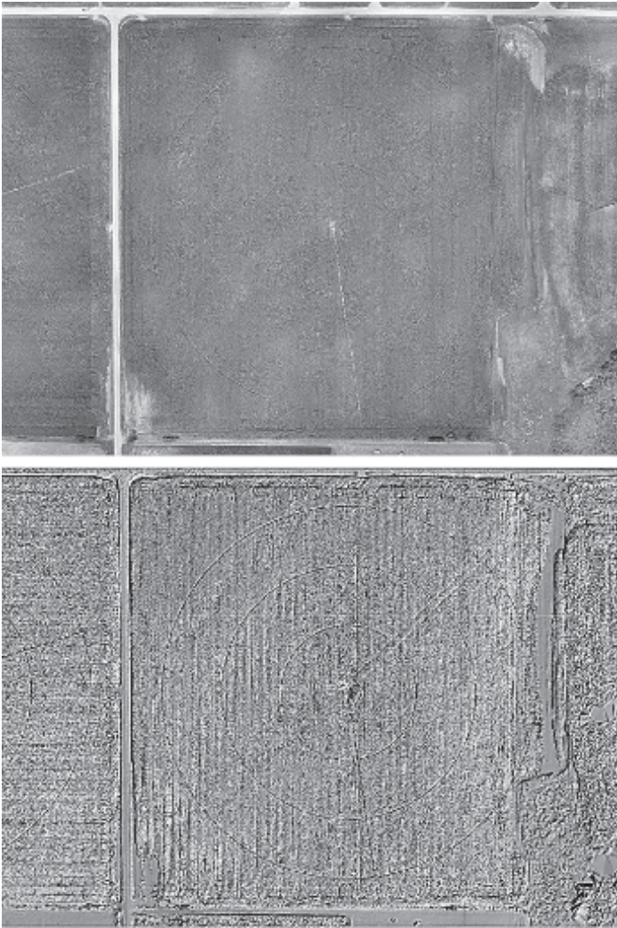
PLATE 8.4 Top: An aerial image of maize obtained using red, green and blue band width cameras mounted on a SenseFly's drone. Bottom: A high resolution Digital Crop Surface Model of the same field obtained, using a low flying drone.
