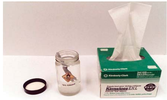
FIGURE 11.4. 120-mL jar with 70% ethanol and orlon wool layer on bottom with forceps, Kimwipes for drying forceps.
