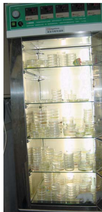
FIGURE 9.3. Temperature-gradient incubation chamber having several closed chambers whose temperatures can be independently controlled.
