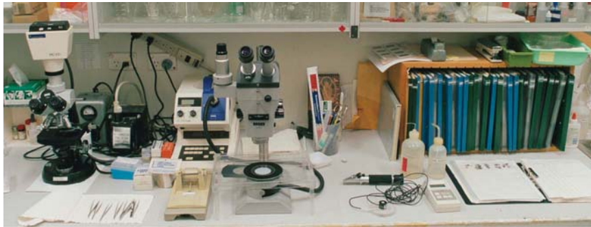
FIGURE 11.5. The arrangement of equipment and materials at the bench for culture transfer and observations. From left to right are shown: Kimwipe dispenser, dissecting tools and label dispenser, compound microscope and camera system, stereomicroscope with fiber-optic illuminator and hand rest, salinity refractometer, Li-Cor 185 meter, polyethylene wash bottles of sterile seawater and Milli-Q water, storage shelf for culture record binders, open binder.
