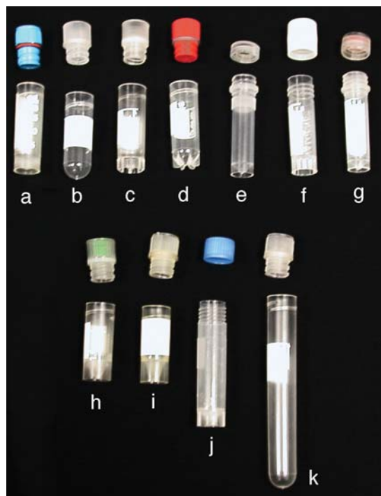
FIGURE 12.2. Plastic cryogenic vials: 1- to 2-mL volumes (a–j) and 5 mL capacity (k). Vials with inside cap threads (a–d, h, i, k) or outer cap threads (e–g, j); gasket molded into the vial (e, g), molded into the lid (f), or as a separate ring (e.g., a); rounded bottom (b, k) or flat bottom and free-standing (a, c–j). Outer vial diameter, labeling surface, colors of lids or lids inserts, transparency, and construction material (e.g., polypropylene, polyethylene) vary.
