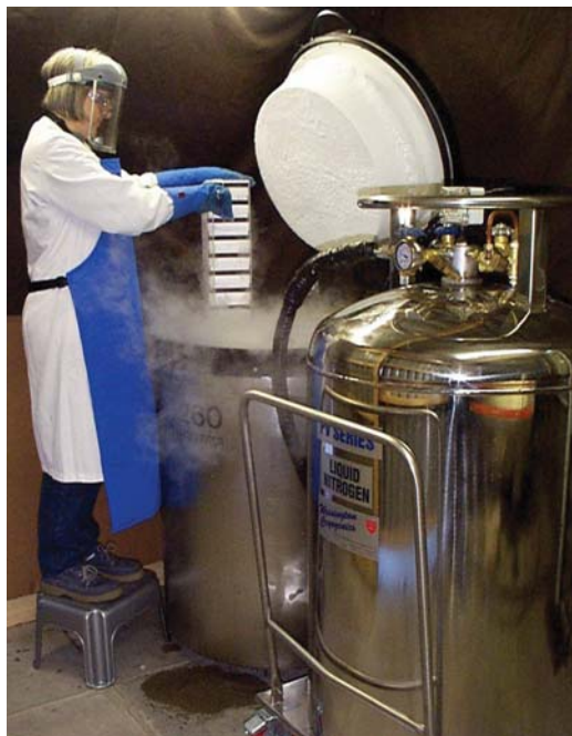
FIGURE 12.6. Removing a vertical storage rack from an automatic-fill storage dewar (left) that is connected to a liquid nitrogen reservoir (right).
