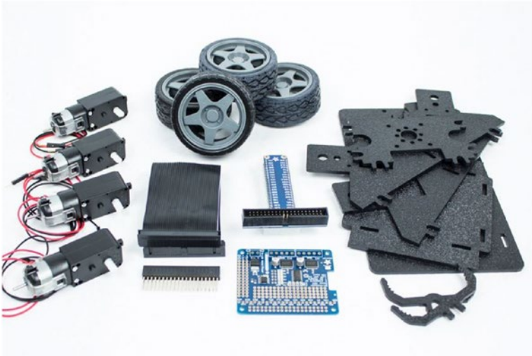
Figure 1-5. Runt Rover chassis parts and the Pi T Cobbler, ribbon cable, motor control hat, and extended header
