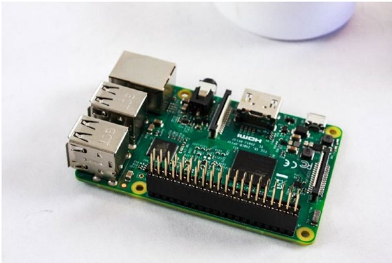
Figure 6-6. Extended stacking header on the Pi's 40-pin GPIO
