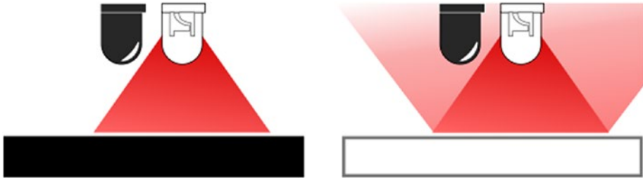
Figure 8-2. Lines and edges can be detected by the difference in reflected light
