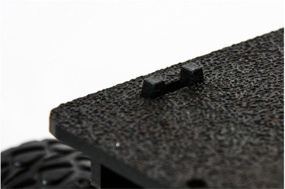
Figure 7-11. Clip protruding from the top plate
