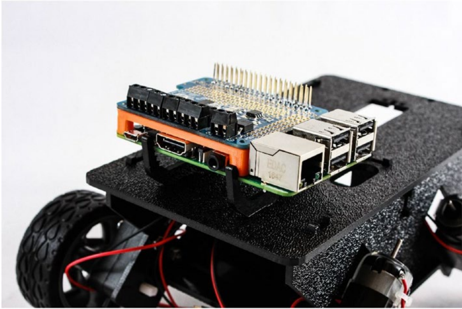
Figure 7-10. Raspberry Pi mounted in the clips
