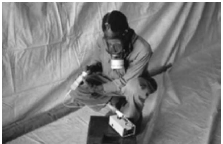
Fig. 7.3 Measurement of phosphine concentration using an electronic meter.
