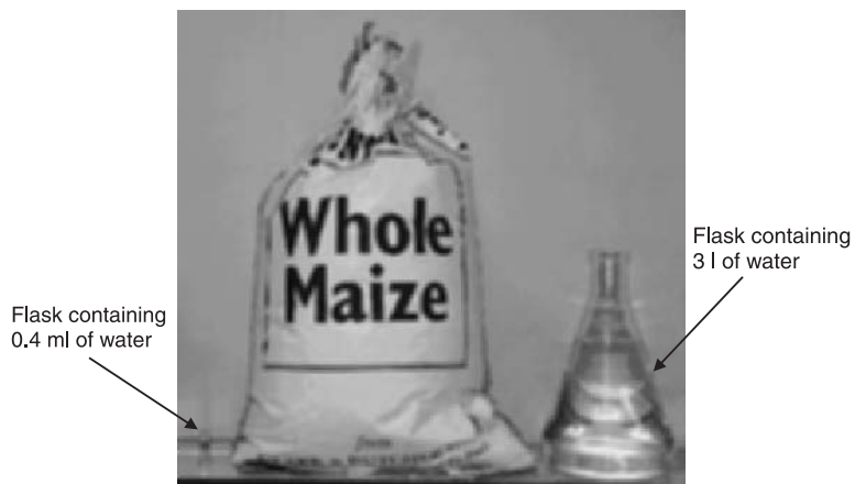
Fig. 3.5 Moisture capacity of maize and air. The picture shows a 25 kg sack of maize. It will typically contain 3 litres of water, shown on the right of the photograph. If the sack contained only air, the air would typically contain around 0.4 ml of water, shown in the tiny flask on the left of the photograph.
