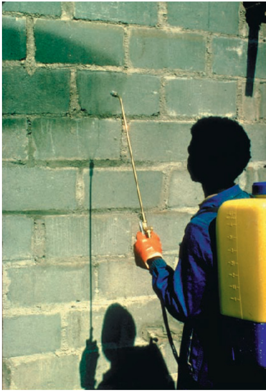
Plate 4 Liquid spray application onto a store structure using a hydraulic knapsack sprayer.
