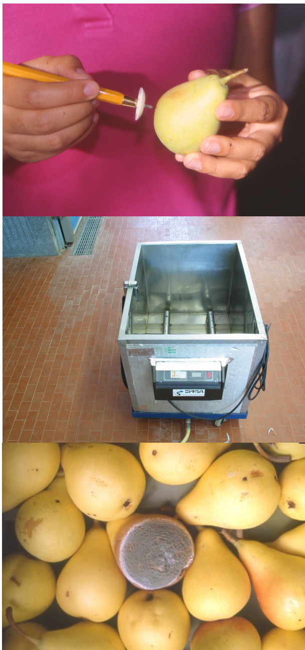
Fig. 4. Wounding of 'Coscia' pears before inoculation with Penicillium expansum (upper), apparatus for water dip at 50 °C (middle), and mould development after shelf life (above) (Schirra et al., 2008b; pictures of the author).
