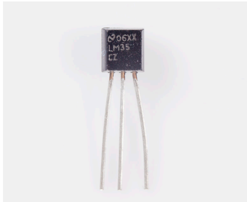
Figure 3-17. LM35 temperature sensor
