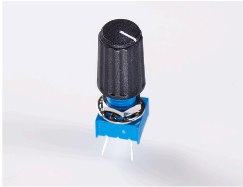
Figure 3-10. Potentiometers can measure rotation
