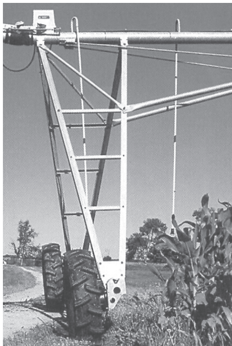
FIGURE 10.5 - The Support towers.
