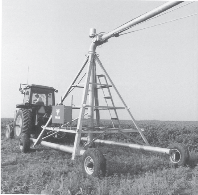
FIGURE 10.8 - Towing the system.
