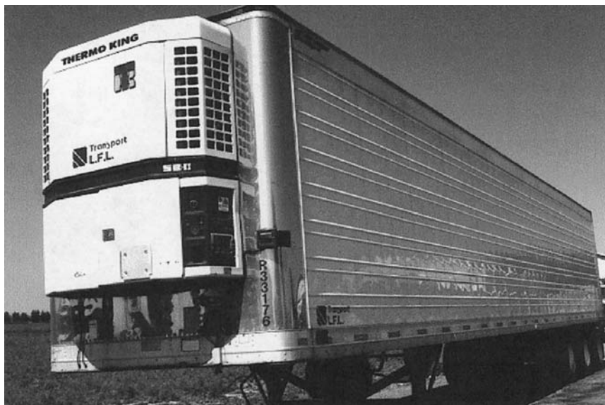
Fig. 3 Nose-mounted refrigeration system used in a semitrailer.
