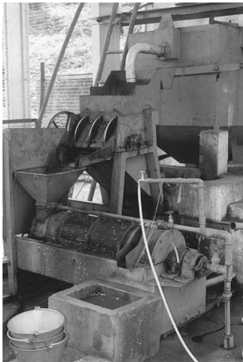
Fig. 4 Pulper cum washer. (Courtesy of Coffee Research Sub-Station, Chettally, Kodagu, India.)
