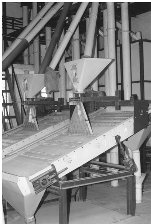
Fig. 11 Peaberry separator. (Courtesy of Chamundi Coffee Curing Works, Mysore, India.)
