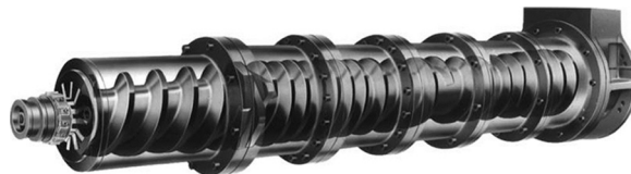
Figure 16.2 A cross-section of a single screw extruder with a segmented worm screw and barrel.
