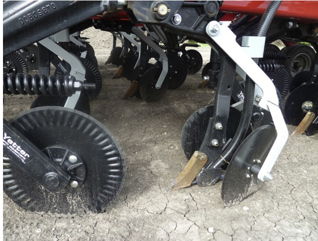
Figure 5.3 Hoe opener with cutting coulter and closing discs.
