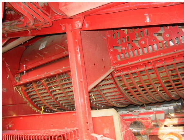
Figure 6.8 Concave around rotor with clean grain augers underneath.
