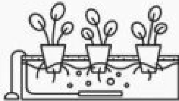
DEEP WATER SYSTEM
