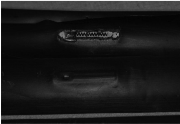
FIGURE 3 Roots penetrating an emitter in the drip-line.
