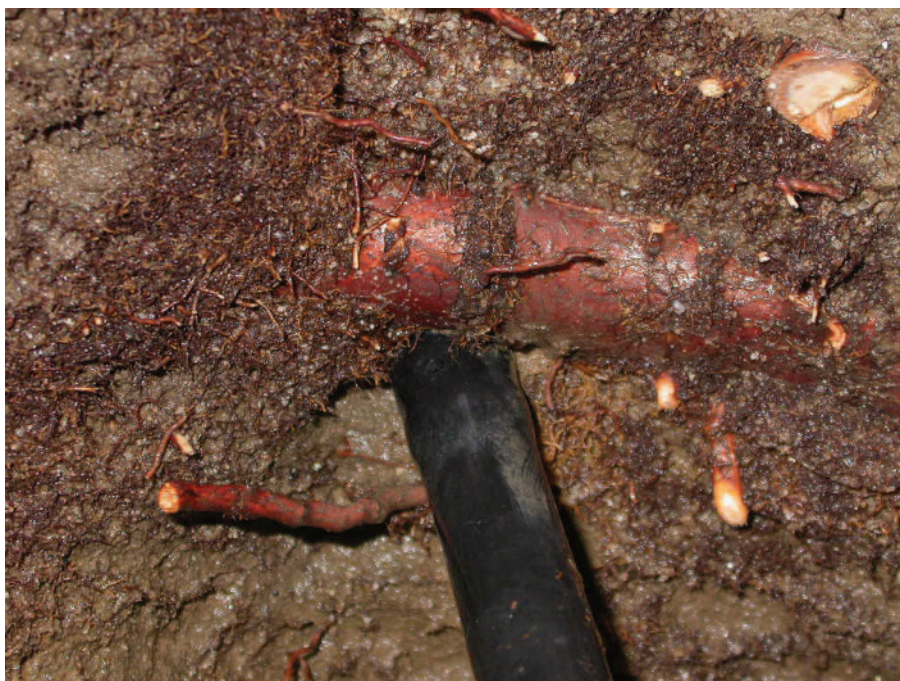
Figure 13.6. Subsurface dripline pinched by peach tree root in California, USA. Photo courtesy of T. Trout, USDA-ARS, Parlier, California.
