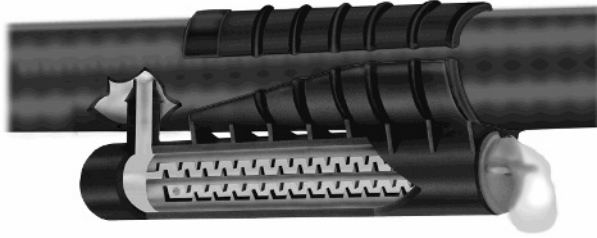
Figure 12.2. Schematic of a turbulent-flow, tortuous-path drip emitter. Courtesy of Bowsmith, Inc.
