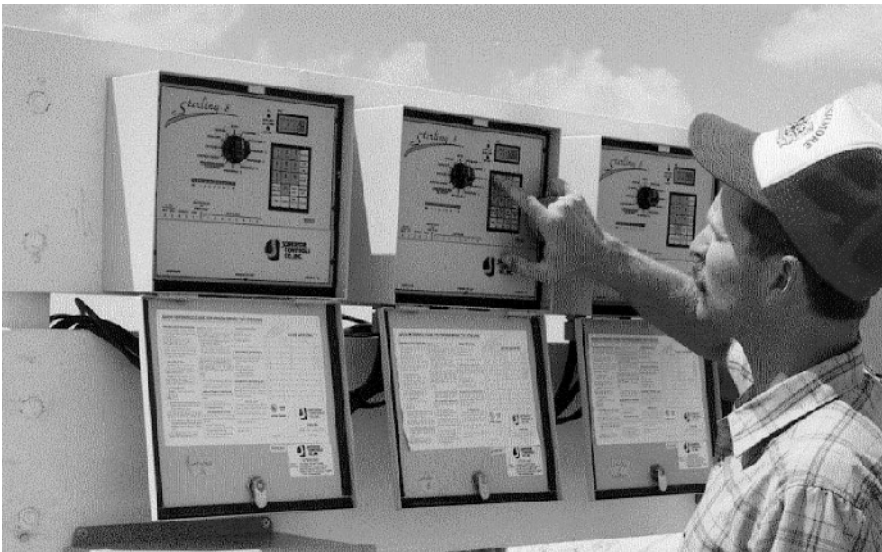
Figure 1.8. Programming an automated microirrigation system. Photo courtesy of Freddie Lamm, Kansas State University.
