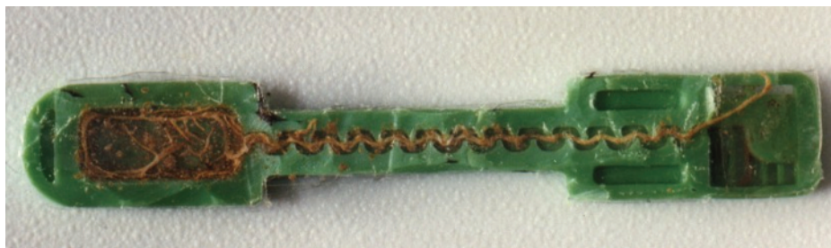
Figure 13.5. A sugarcane root entering the outlet chamber on the left can intricately grow through the labyrinth and the emitter inlet filter on the right and into the dripline. Photo courtesy of Z. Golan, Plastro Irrigation.
