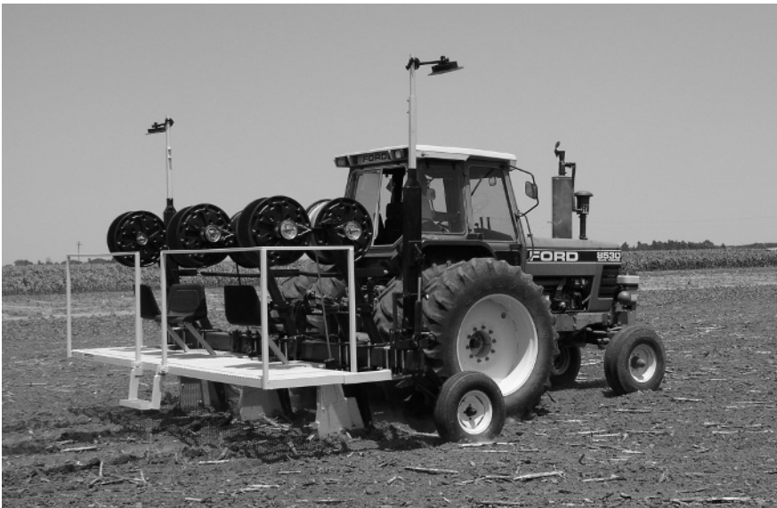
Figure 13.21. Tractor-drawn SDI installation implement installing dripline in Kansas. Courtesy of F. R. Lamm, Kansas State University.
