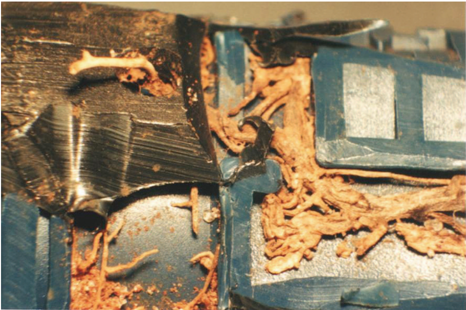
Figure 13.4. Single coffee plant root entering an emitter can enlarge into a large root mass once inside the emitter and dripline. Photo courtesy of Rubens Duarte Coelho, University of Sao Paulo, ESALQ / Brazil.
