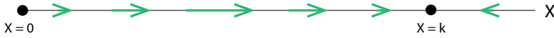
Figure 1.36: The vector field for the logistic equation, X' = rX(1 - \frac{X}{k}) , with r = 0.2 and k = 100 .
