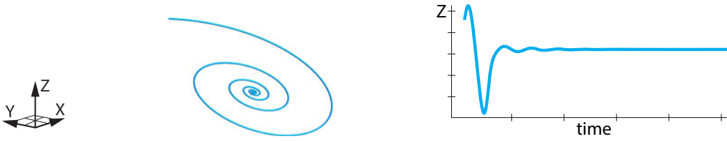
Figure 5.23: For low values of b_1 , the system has a stable equilibrium point of spiral type.
