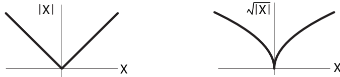
Figure 2.15: The functions |X| and \sqrt{|X|} have corners or cusps at X = 0 and are not differentiable there.
