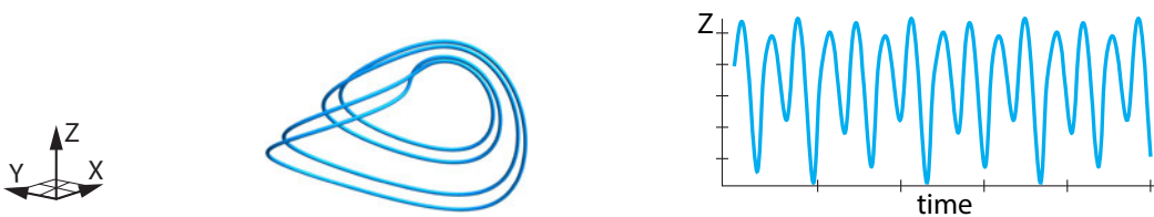
Figure 5.26: Still further increases in b_1 cause a second period-doubling bifurcation, to an even more complex periodic rhythm.
