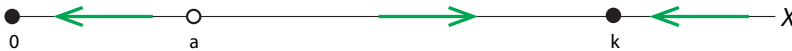
Figure 3.10: By drawing representative change vectors on state space, we can easily see the stability of the system's equilibrium points.
