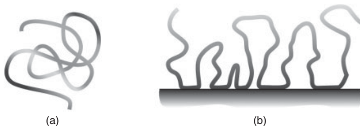
Figure 1.12 Structure of a coiled polymer (a) in solution and (b) adsorbed onto a surface.
