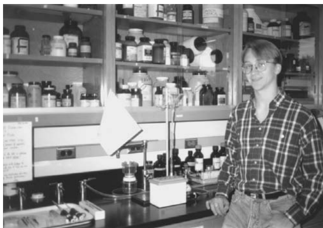
FIGURE 8.6 Leland Cseke is shown with the C18 Sep-Pak™ column (lower center) used in our laboratory to partially purify yew ( Taxus spp.) plant extracts in preparation for high-performance liquid chromatography analysis of taxane-type diterpenes found in these plants.
